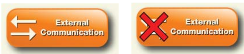
Figure 25-10: External Communication Status Indicator (Normal and With Connection Problems)
